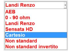
Exclusively on Omegas 194 units (616,448,000) and Omegas 198 (616 469 000) you must select "NON STANDARD" as a sensor and manually enter values as below:
